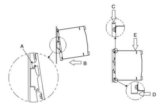
DIN-rail mounting of POWER SUPPLIES
